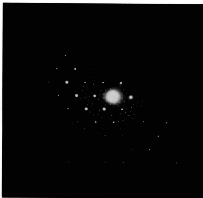
Fig.3. CuSe: one twin component predominating. Orientation [31\bar{4}T] .
